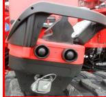
Picture 11: frame and basket connectors for wired remote control.
