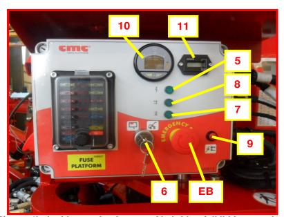
Picture 4b: ignition station in case of hybrid or full lithium version.
