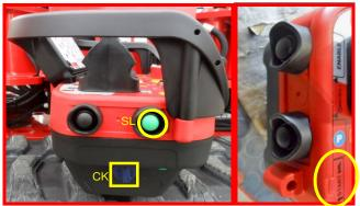
Picture 7: start/link button on radio control.
