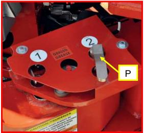
Picture 18: setting operations on stabilizers pin.
