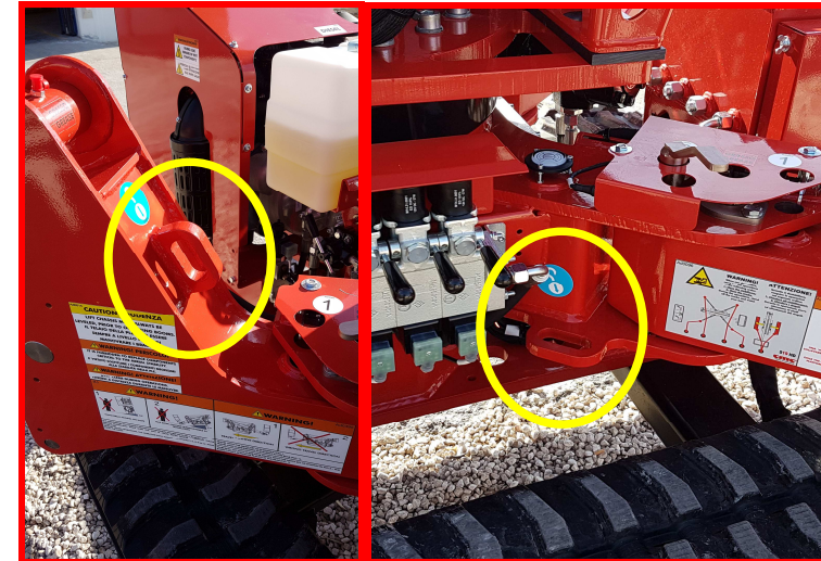
Picture 16: hooks for sling and lifting.
