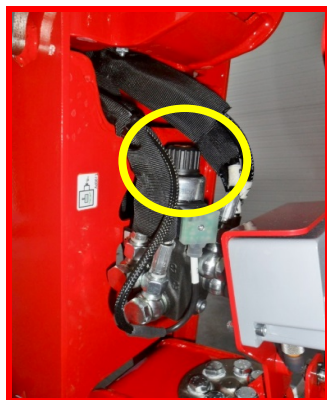
Picture 24: valve cursor for basket centering.
