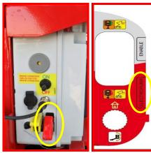
Picture 29: electropump activation buttons.
