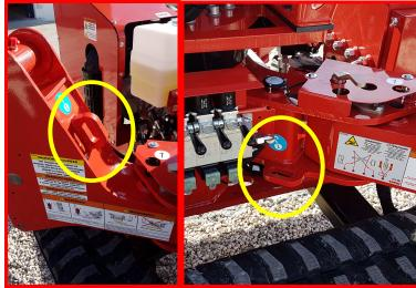
Picture 16: hooks for sling and lifting.
