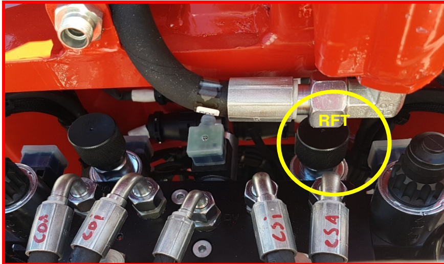
Picture 26: right filters bench tap.
