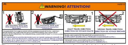
Picture 43: warning for machine travel, on left/right side of frame.
