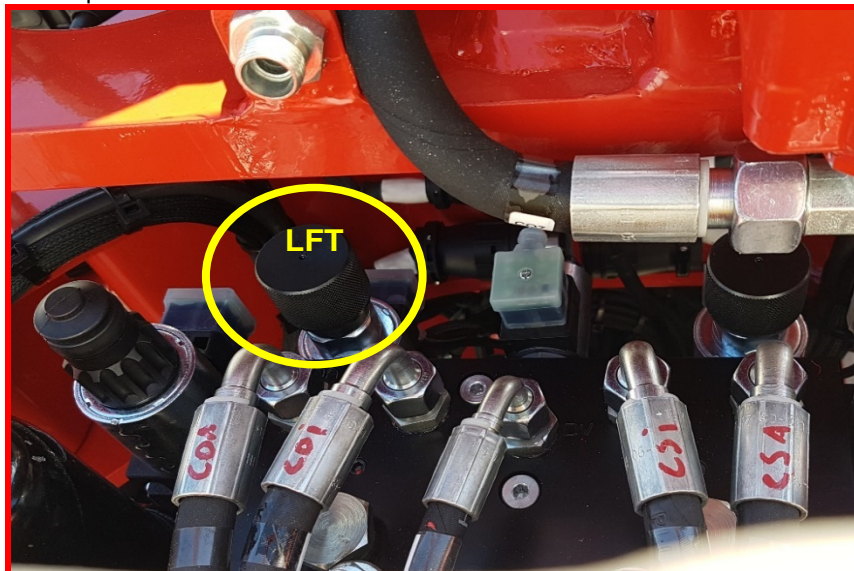
Picture 22: left filters bench tap.
